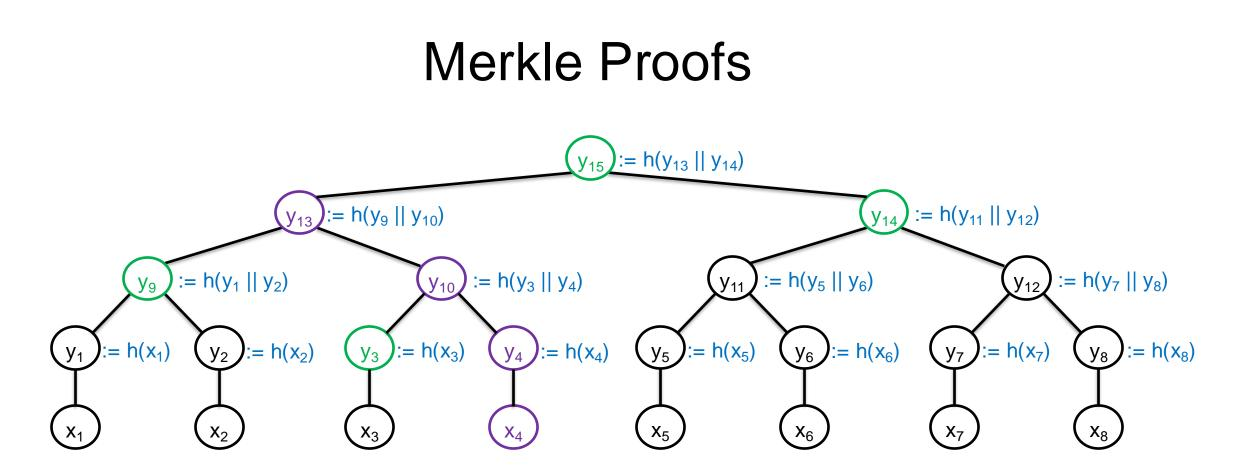
To prove that  $t = x_4$ : exhibit siblings along root-leaf path:  $y_3$ ,  $y_9$ ,  $y_{14}$ . To verify: compute  $z_4 = h(t)$ ,  $z_{10} = h(y_3 || z_4)$ ,  $z_{13} = h(y_9 || z_{10})$ ,  $z_{15} = h(z_{13} || y_{14})$ , check that  $z_{15} = y_{15}$ .
