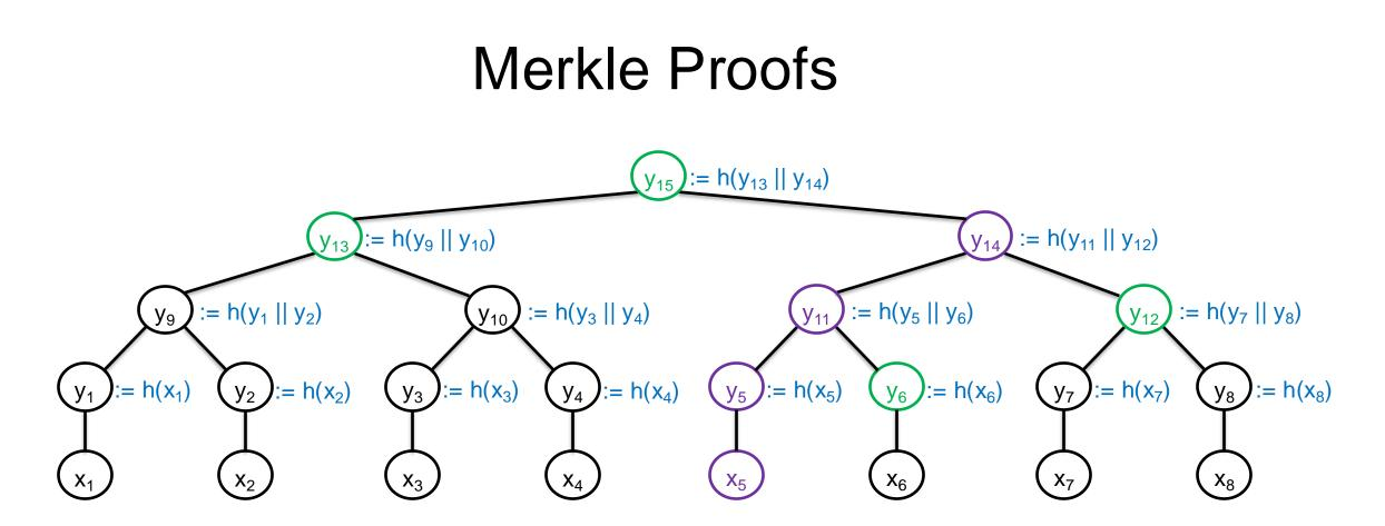
To prove that  $t = x_5$ : exhibit siblings along root-leaf path:  $y_6$ ,  $y_{12}$ ,  $y_{13}$ . To verify: compute  $z_5 = h(t)$ ,  $z_{11} = h(z_5 || y_6)$ ,  $z_{14} = h(z_{11} || y_{12})$ ,  $z_{15}=h(y_{13} || z_{14})$ , check that  $z_{15}=y_{15}$ .
