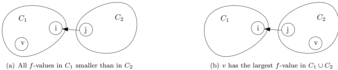
Figure 7: Proof of Key Lemma. Vertex v is the first in C_1 \cup C_2 visited during the execution of DFS-LOOP on G^{rev} .
