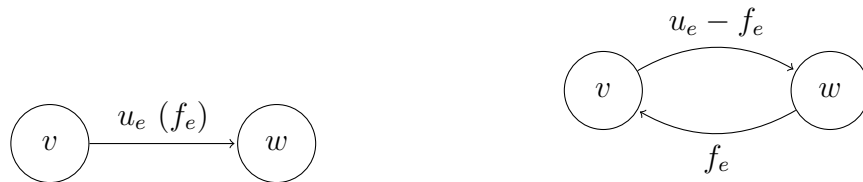
Figure 4: (a) original edge capacity and flow and (b) resultant edges in residual network.
